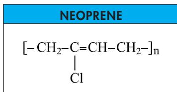
Neoprenes are homopolymers of chlorobutadiene with service temperatures from  $-65^\circ$  to  $300^\circ\text{F}$ . This material is unique in its limited resistance to petroleum products, ozone and weathering, and relatively low cost. Neoprene typically has a 20% premium over the cost of Nitrile oil seals.
